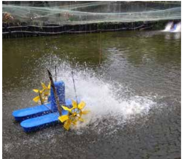
Fig. 17. Paddle wheel aerator installed at brood fish management pond
