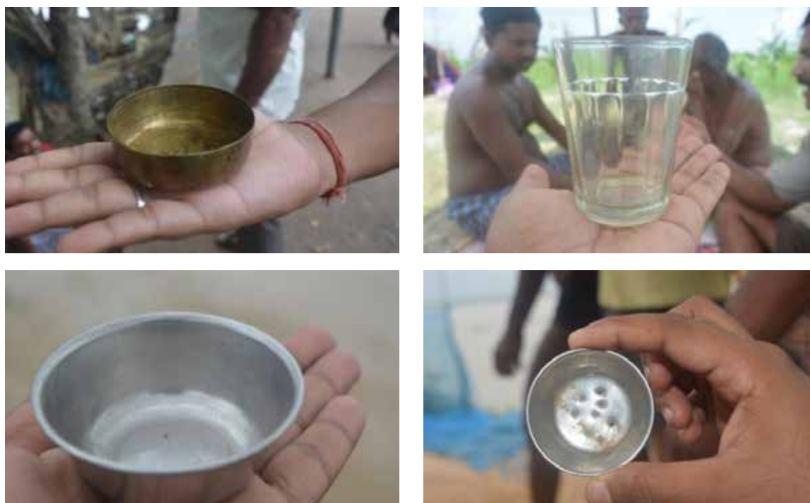
Fig. 97 (A-D) Different fish spawn measuring devices used in river Ganga during the collection period
